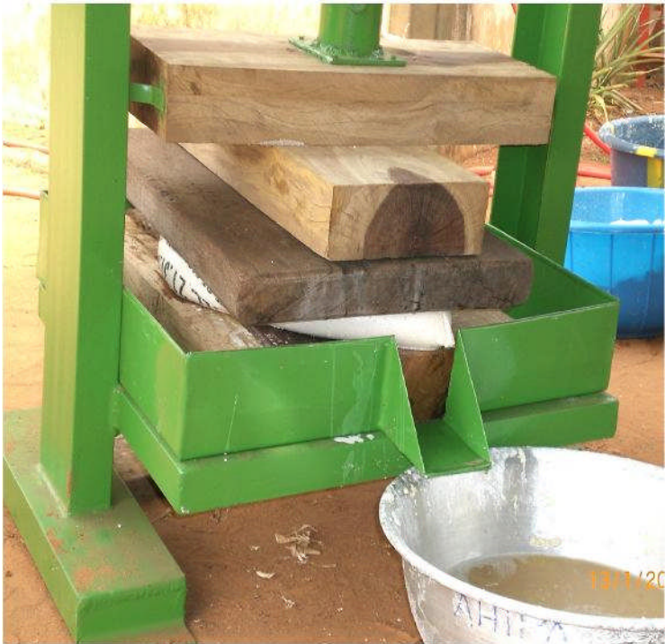
Figure 7: Pressage de la râpure de manioc
